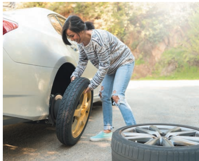
Figure 8-21 A spare tire is usually smaller and less capable than a full-size tire
