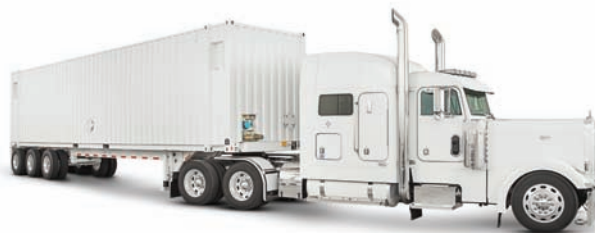
Figure 3-5 Snowmobile can transfer up to 100 PB per trip
