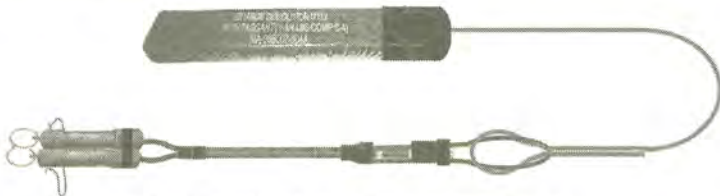
Figure 19-4. Primed Explosive Charge and Firing System.
