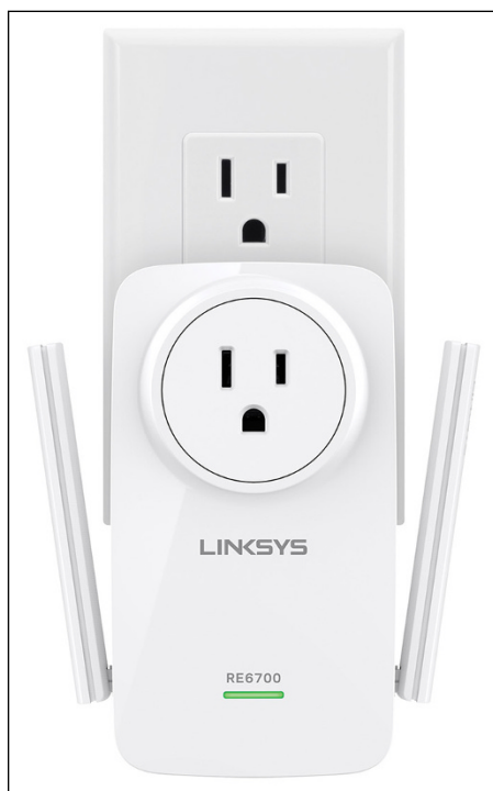
FIGURE 2-8: A wireless repeater such as this one from Linksys can help increase the range of your wireless network.
