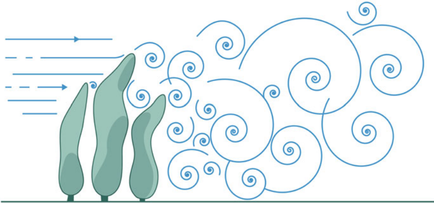
Fig. 5.4 Schematic representation of several vortices produced by a complex family of boundary obstacles. Picture by Claudia Flandoli
