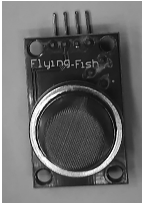
FIGURE 11.10 MQ-2 gas sensor to measure the gas concentration in the atmosphere.
