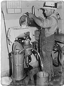
The hand-operated cream separator was a valued possession for early immigrants. They were able to sell cream from their milk cows for real money.
