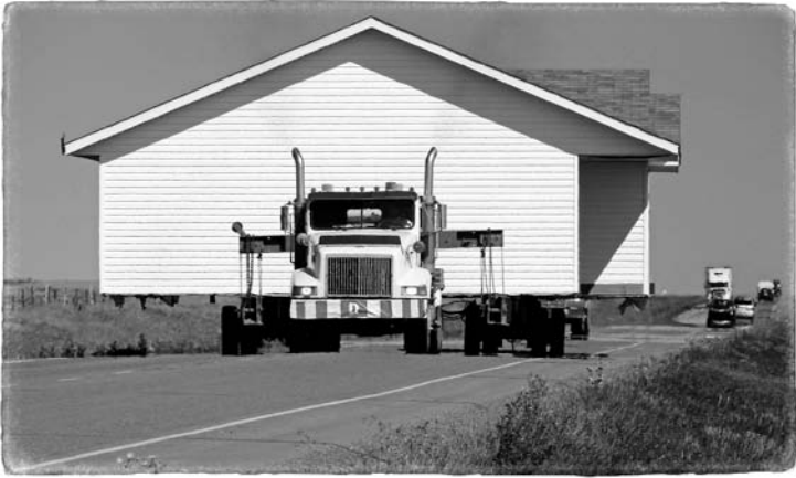
These days it is a common sight to see a section of a double-wide manufactured home being transported from factory to building site.
