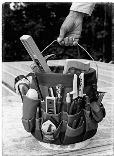
The 5-gal. bucket became the "toolbox" of choice for most production framers.
