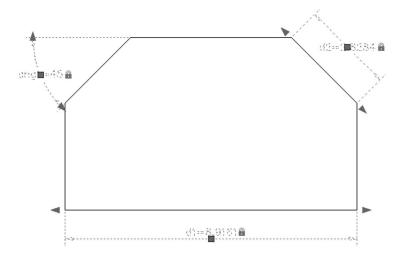
As you can see there are grips at the middle of each dimensional constraint that will move the whole block back and forth. The other two arrows will stretch the dimensional constraint, and hence stretch the object by itself. Dimensional parameters have their own grips depending on the type.
