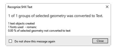
An MTEXT will be created accordingly. AutoCAD will create a new text style holding the name of the font and assign the text to it.
