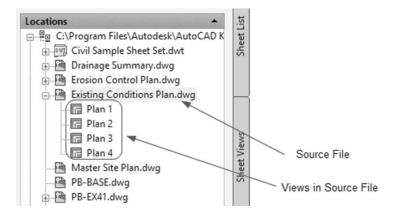
The Model View tab contains the AutoCAD files named source files, which contain the views which will be used in the first method of sheet sets (user will be using the drag-and-drop method to insert these views as an external reference to the current file).
