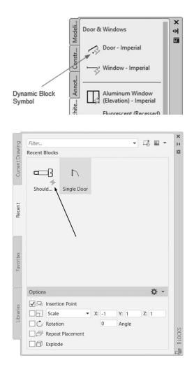
Dynamic blocks are very handy tools to help you to finish drawing production faster and with less mistakes, reducing the number of blocks to work with.
