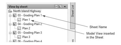
Using the Model Views tab, if you dragged and dropped a model view, then the Sheet View tab will show the name of the sheet and the name of the view inserted in it.
