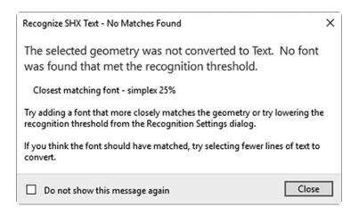
If you want to convert more geometry to fonts in the PDF import, go to **Insert** tab, locate **Import** panel, click **Recognize SHX Text** button:
