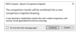
Read the message carefully which states that the comparison results will be combined into a new comparison snapshot drawing. Click Continue, and either accept the default name of the new drawing, or type the new name.
