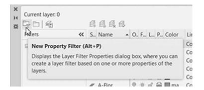
• Or, using the Layers panel, use the first list, and click the New Layer State button:
