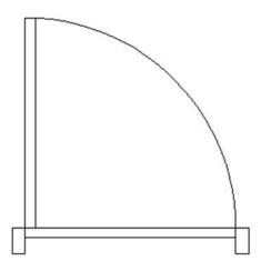
**11.** Add a Visibility parameter, selecting the upper left part of the door to be the location of the parameter. Note how the Visibility panel was turned on
