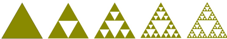
Figure 14: Sierpinski gasket antenna through five stages of growth.
