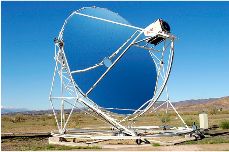
FIG. 7.10 Solar dish with center-mounted Stirling engine [17].
