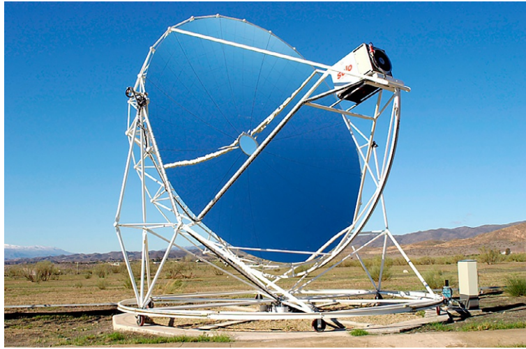
FIG. 7.10 Solar dish with center-mounted Stirling engine [17].
