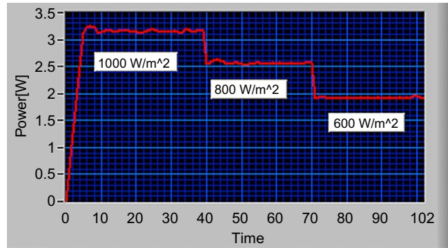
FIG. 5.52 Output power of incremental conductance algorithm under varying solar irradiance [15].
