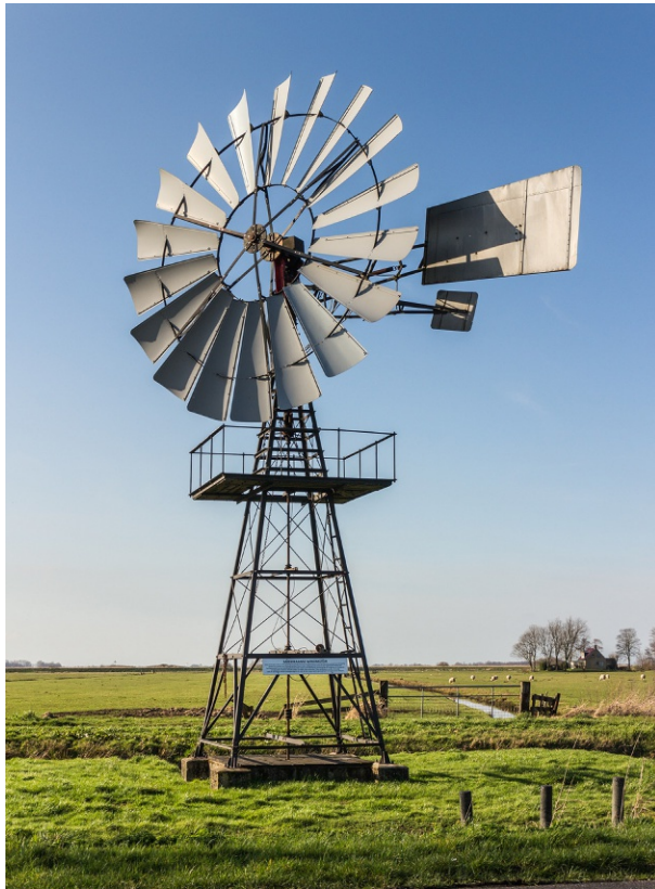
FIG. 6.6 Multibladed horizontal axis wind turbine. Source: Wikipedia.
