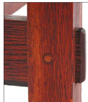
Pegged mortise-and-tenon joint on a Stickley oak side table.
