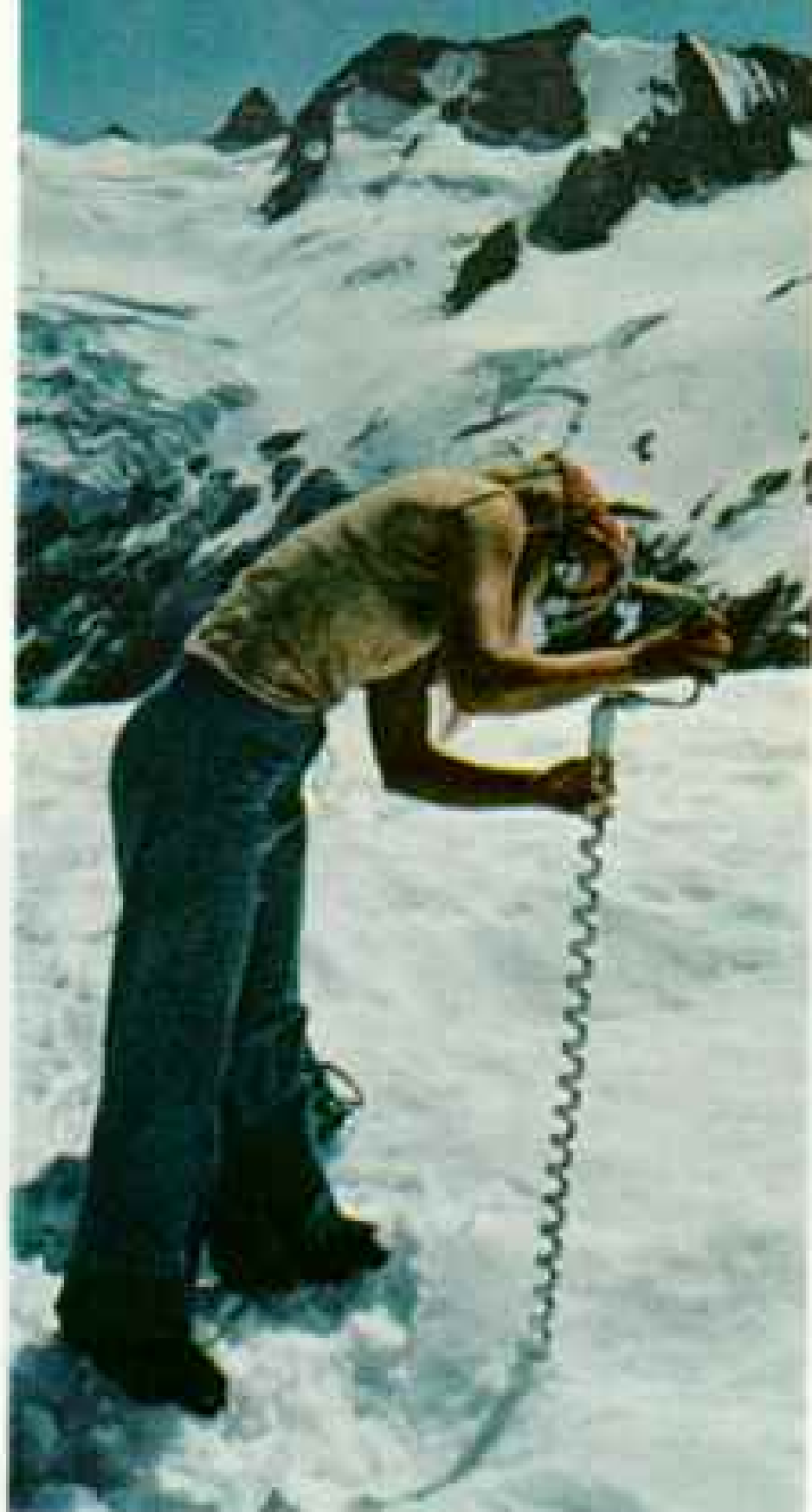
Tracking a glacier in the Cascade Range, U. S. Geological Survey worker Mindy Brugman bores a hole for a marker stake. South Cascade Glacier advances about three feet each month.
