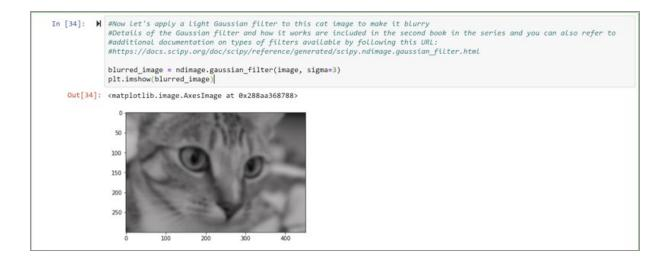
And now, let's make it blurry by increasing the sigma value for the Gaussian filter:
