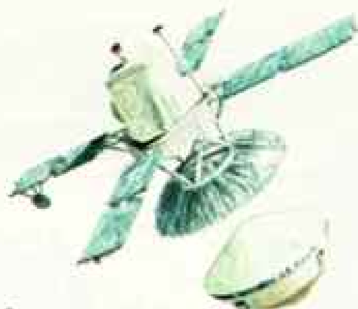
2 Orbiter releases lander inside aeroshell
