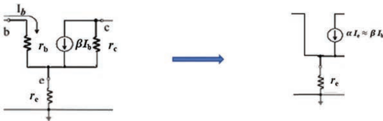
Figure 6.7 Simplified BJT r parameter equivalent circuit
