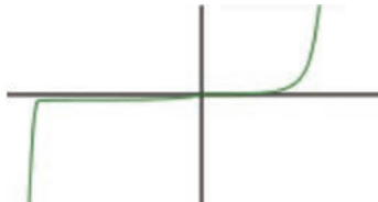
Figure 1.25 I-V curve of a real diode
