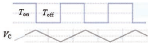
Figure 11.11 Waveforms of a step-down voltage regulator
