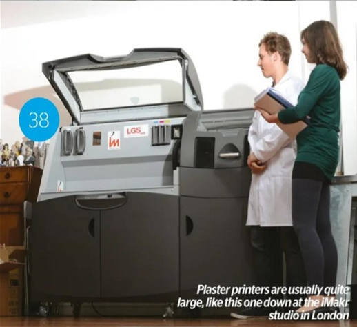
The printing method itself is powder-based, as with SLS printers
