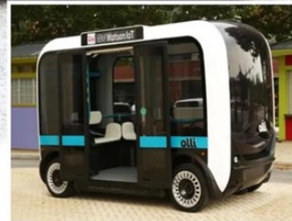
Olli is the world's first 3D-printed self-driving shuttle. It can transport up to eight people at once
