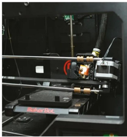
Load your filament correctly to avoid it tangling and twisting
