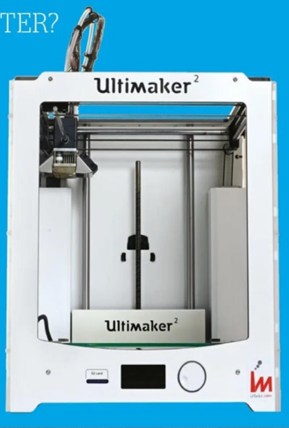
The extruder itself is attached to something called an x carriage
