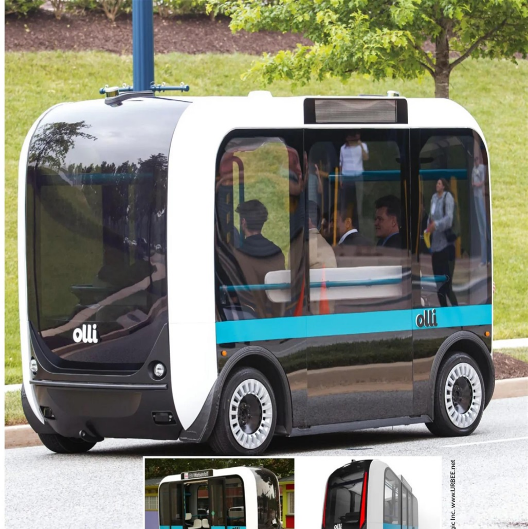
Olli is the world's first 3D-printed self-driving shuttle. It can transport up to eight people at once
