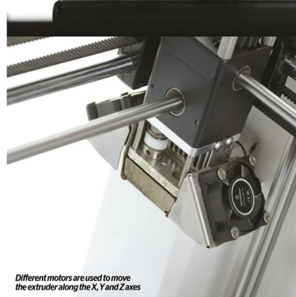
The filament to build up the print comes through the extruder
