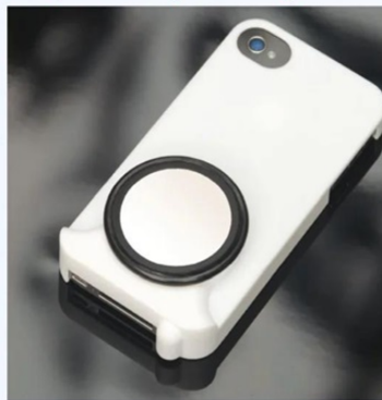
The Steth IO prototype and how it would work as very accessible stethoscope
