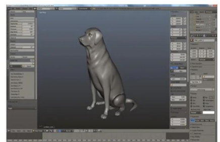
ABOVE The 3D Print toolbox will highlight regions with overhangs, along with a number of other printability issues
