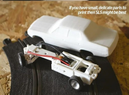
SLS is also suitable for models where a high level of accuracy is required
