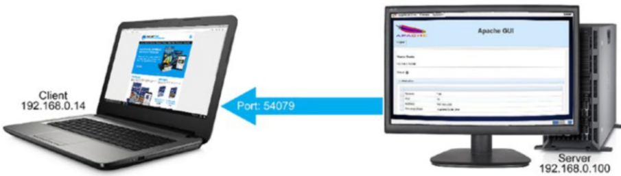
Figure 1-32. Connection Assigned Port Number
