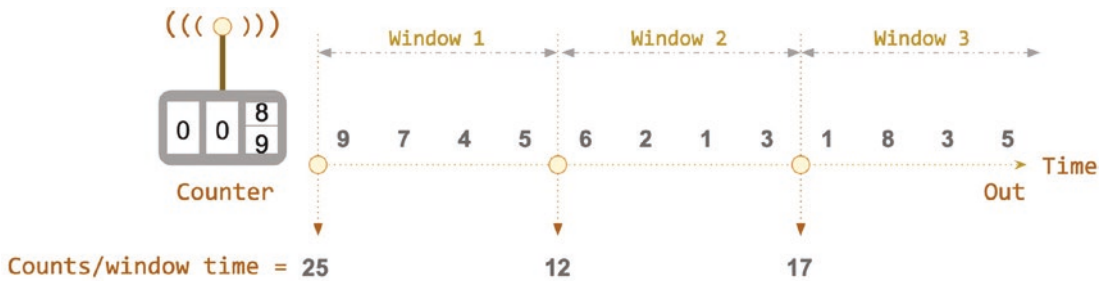
Figure 9-4. Example of temporal window to count events per window time
