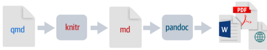
Figure 28-4. Diagram of Quarto workflow from qmd , to knitr , to md , to pandoc , to output in PDF, MS Word, or HTML formats.
