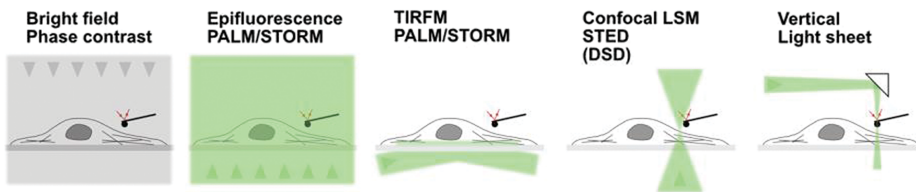
Figure 3.8.1: Types of illumination patterns used in current AFM/optical correlative microscopy.
