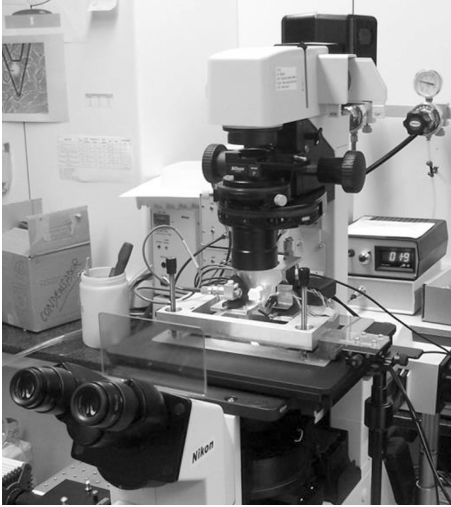
Figure 3.1.1.6: Home-built AFM coupled to an optical microscope (Rico, 2006).
