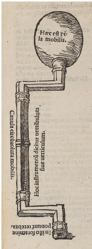
Fig. 3.14 Drill with a rotating handle. (From: J. Berengario da Carpi. De Fractura calvae sive Cranei , Bologna, Hieronymus de Benedictis, 1518)
