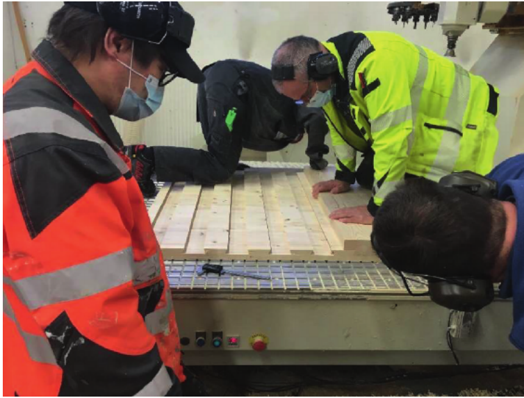
Figure 9. Manufacture of dovetail massive wood board element at Vocational College Lapland (Ammattiopisto Lappia), Kemi, Finland (photo by Hüseyin Emre Ilgım).
