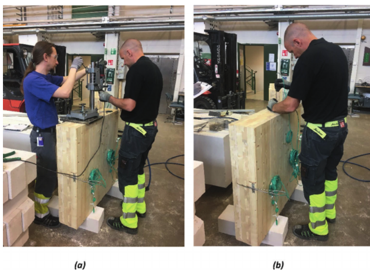
Figure 10. Preparation of dovetail specimens for fire resistance test at Tampere University Fire Laboratory, Tampere, Finland. (a) Drilling and (b) thermocouple insertion (photos by Hüseyin Emre Ilgın).
