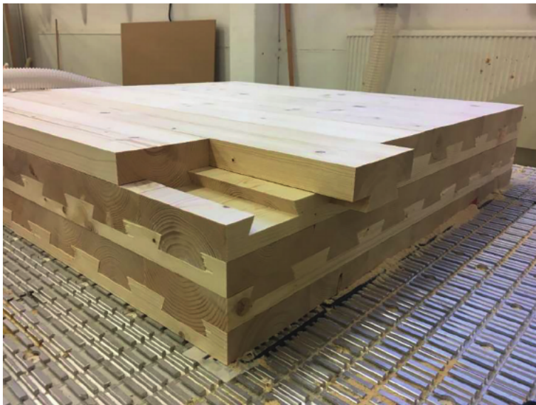
Figure 5. Test specimen of adhesive- and metal fastener-free dovetail wood board element (photo by Hüseyin Emre Ilgin).
