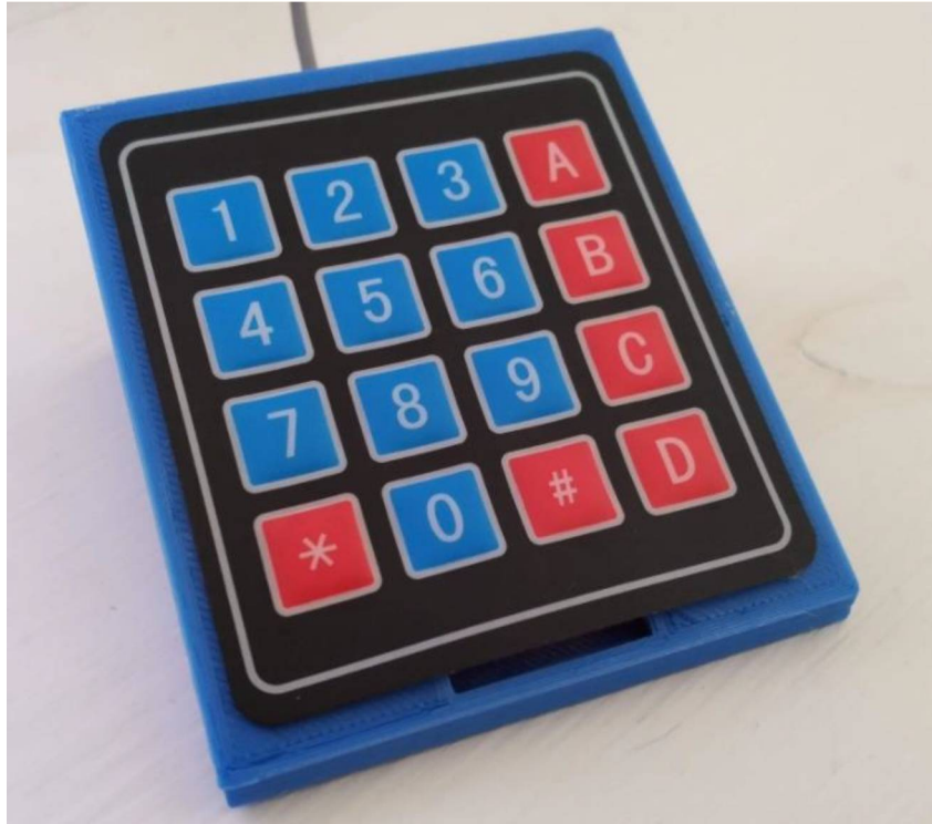
Figure 17: A DIY keypad to control applications. Source: Github
