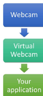
Figure 9: Video flow when a virtual webcam is used.
