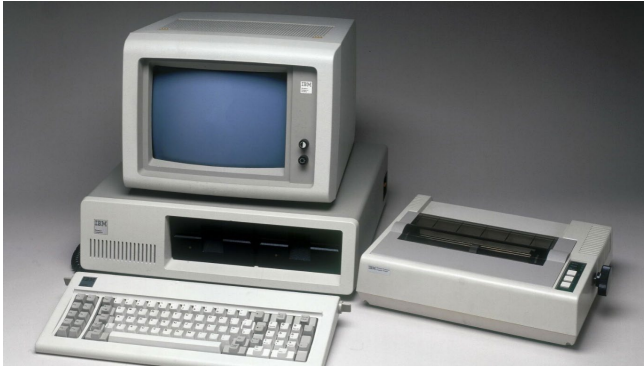
Figure 2.9. The original IBM personal computer (1981) utilized an Intel 8088 microprocessor.
