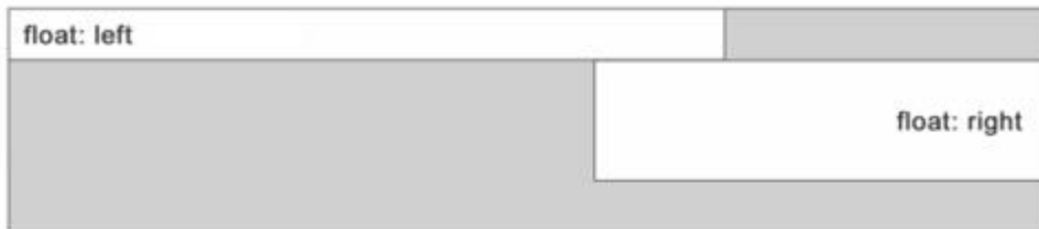
Figure 89: If the total sum of two floating element's is greater than parent's width, one of them will be blocked by the other and skip over to the next row.
