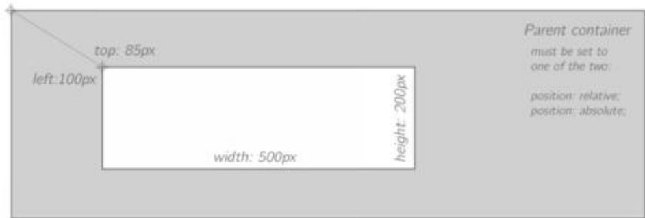
Figure 62: The parent container must be explicitly set to either position: relative or position: absolute in order to use a child element within it that also uses position: absolute align.
