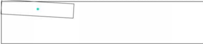
Figure 134: Rotating an element around its center using rotate( angle ) , where angle is an angle between 0 and 360 degrees, with "deg" appended.
