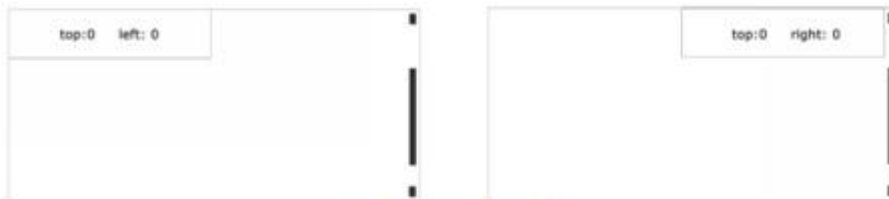
Figure 22: Using position:fixed works the same as position:absolute except that the scrollbar will not affect its position.
