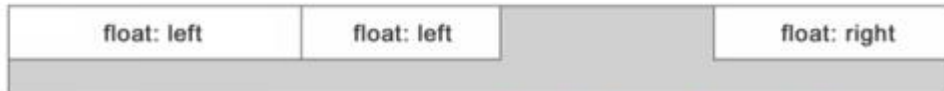
Figure 88: Blocking elements with float:left and float:right appear on the same row, as long as the sum of their widths is less than the width of the parent element.
