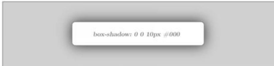
Figure 66: Here box-shadow is used to add a shadow around a wide element. It takes the same parameters text-shadow does, for example: box-shadow: 5px 5px 10px #000 (x and y offset, radius of the shadow, and shadow color .)
