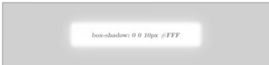
Figure 68: Using bright colors with box-shadow property it is possible to create glowing effect around HTML elements.
