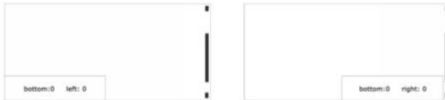
Figure 23: The origin point can be any corner of the element, depending on which property pair that was used ( top & left , top & right , bottom & left or bottom & right ).
