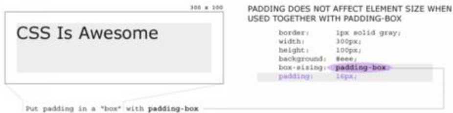
Figure 12: The padding-box value puts padding on the inside of content box. Now, the original dimensions are retained but the content is still padded.
