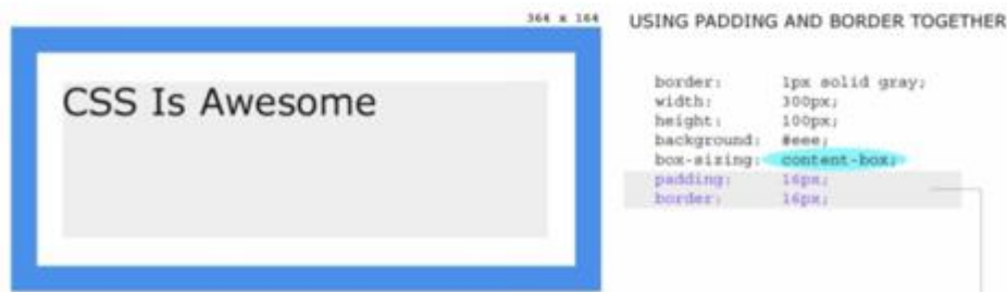
Figure 13: Here we overwrite the original value of border: 1px solid gray from previous example to border: 16px and together with padding: 16px the original width and height of the element are now padded by an extra 32px pixels on each side, adding a total of 64px to each dimension of the element.
