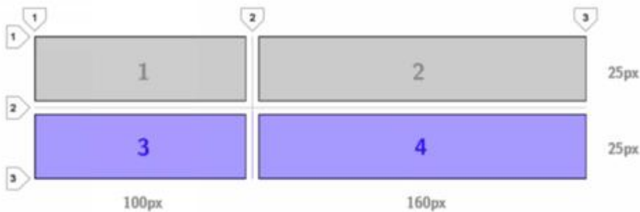
Figure 182: Adding more items into a CSS grid whose row template does not provide enough room to place them will automatically extend the CSS grid to open up more space. Here items 3 and 4 were added to previous example. But the grid-template-columns and grid-template-rows properties provide a template only for 2 items maximum.
