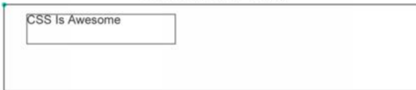
Figure 133: Instead of using top and left properties, we can use transform:translate(30px,10px) to move the element on its X and Y axis.
