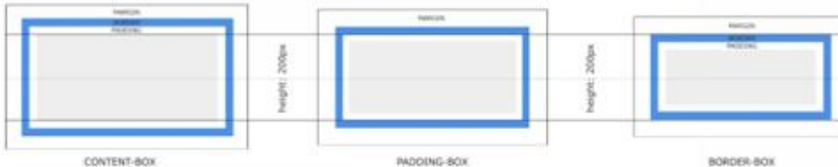
Figure 9: Note that the value 200px of the height property of the element does not change, but its physical dimensions do, based on box-sizing: [content-box|padding-box|border-box]
