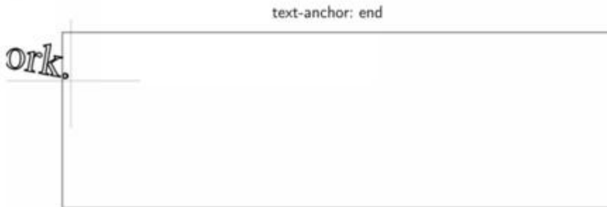
Figure 59: Setting text-anchor to end to offset center of rotation to the very end of the text block. We'll see similar behavior on CSS transform property that can be used to rotate entire HTML elements and text within them.
