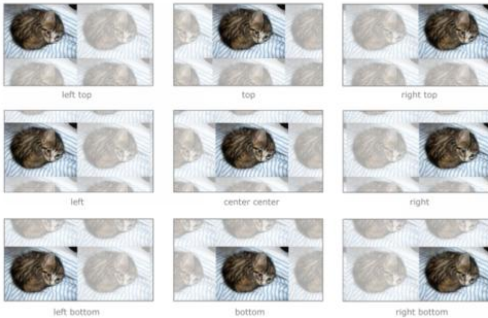
Figure 120: background-position-x and background-position-y are supplied the following values to create any of the background positioning patterns: left top | top | right top | left | center center | right | left bottom | bottom | right bottom .
