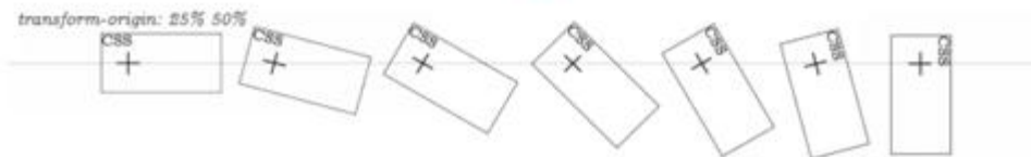
Figure 144: The rotation origin doesn't have to be in the middle or at the corners of the element. It can be anywhere.
