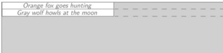
Figure 83: Centered text ( text-align:center ) inside two blocking elements with width set to 50 % of the container. Note, that while blocking the entire row of the parent element, the content area only stretches up to 50 % of its width. A blocking element is not defined by the width of its content.
