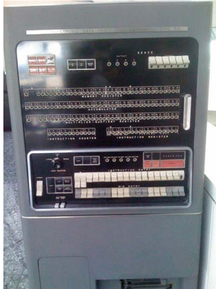
Figure 5.9. The front panel of an IBM 701 computer, which was debuted in 1952. The contents of numerous registers are displayed by lights in the center. The instruction counter is located in the lower left corner.
