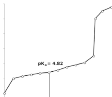
Figure 6.5. Titration A weaker monoprotic acid is titrated with a stronger base. Around the pK_a , a buffering area is created (4.82). The Henderson-Hasselbalch equation describes the pH at any specific spot.
