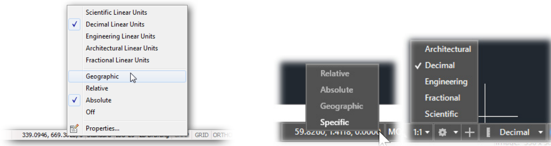
Left: Accessing units formats from the status bar in BricsCAD; right: AutoCAD requiring two status bar buttons
