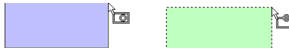
BricsCAD uses colors and icons to report the style of a windowed selection: Left: Making a windowed selection; right: Making a crossing selection.
