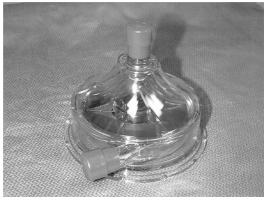
Figure 12.2 Centrifugal Pump, Bio-Medicus Bio-Pump consists for valveless rotator cones, which are made to impart a circular motion to the blood, generating centrifugal force, pressure, and flow.
