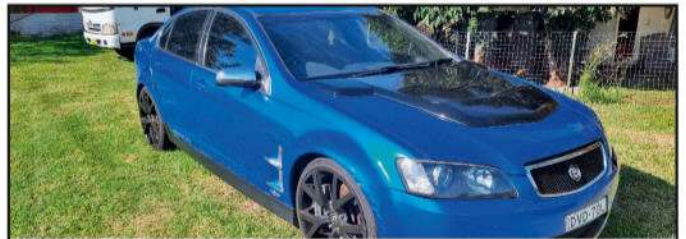
HSV SENATOR SIGNATURE E2 2009, 2009 HSV senator walkinshaw has 50,000kms on the clock, second owner, 6.2l LS3, has been upgraded at walkinshaw performance in Sydney with their stage 3 performance package with upgraded cam, lifters, valve springs, double row timing gears and chain, intake, full stainless exhaust system by walkinshaw true track lsd diff upgrade and 3:45 gear ratio under drive pulley kit and full tune to 330 rkw, front bumper has been removed and repaired and callipers and discs are not with the car, DVD70L. NSW. DIY1231960. 0450 544 789. $38,000
