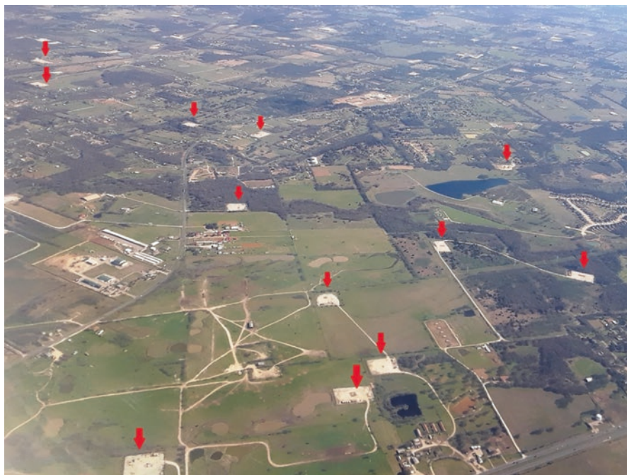
Fig. 7.2 Closely-spaced Barnett Shale drill pads (arrows) visible southwest of DFW Airport. (Photographed in 2019 by Dan Soeder)
