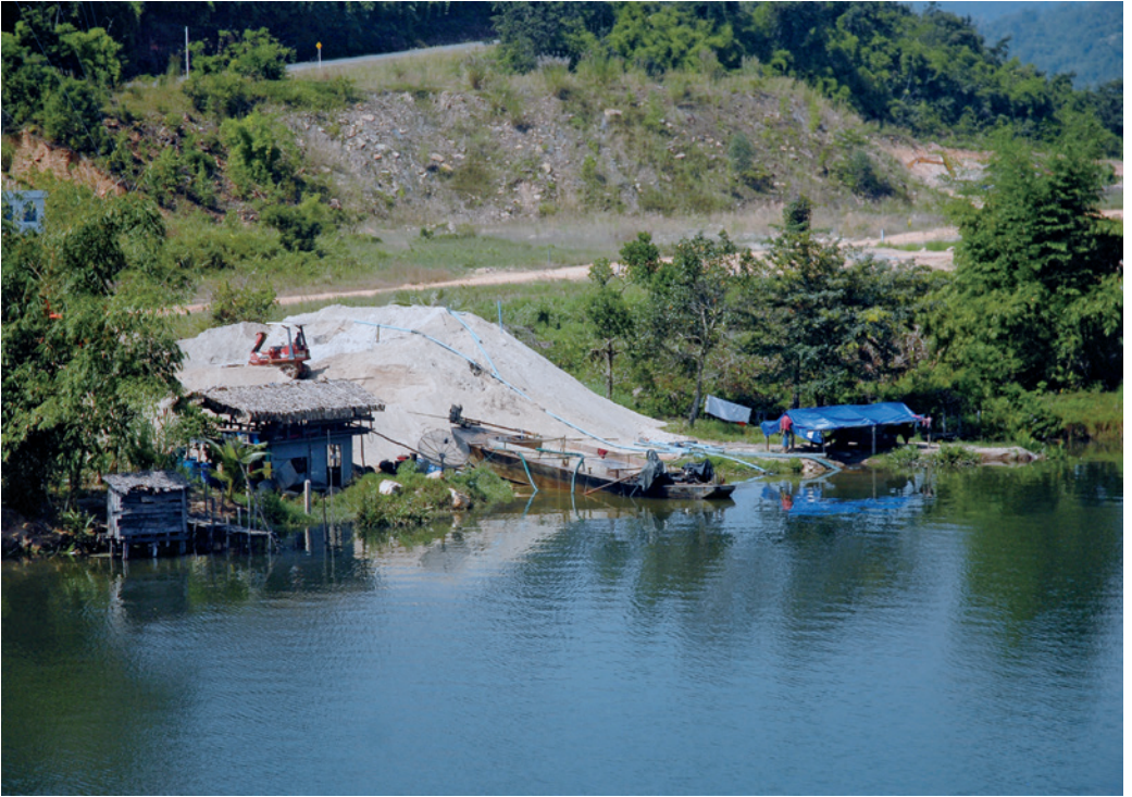
FIG 5.3B A small sand-processing plant on the bank of the Tatai River, Cambodia. Small boats and dredge barges off-load sand that will be trucked or barged to the river mouth for export on sea-going barges. In 2011, the destination was Singapore. Photo © Robert Tyabji Hoorob, Creative Commons CC BY-NC-ND 2.0.
