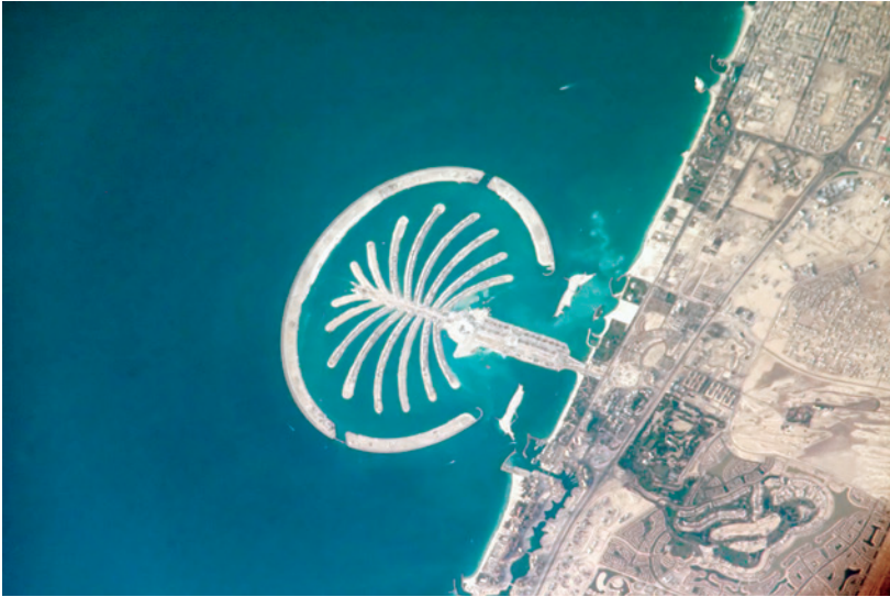
FIG 8.7 Oil-rich Dubai has constructed the world-famous Palm Jumeirah islands using ninety-four million cubic meters of sand dredged from the Persian Gulf. The dredging suspended fine sediment in surrounding waters and killed the local ecosystem, including living coral reefs. View from the International Space Station. Photo by Expedition 10 Commander Leroy Chiao, 2005, NASA.
