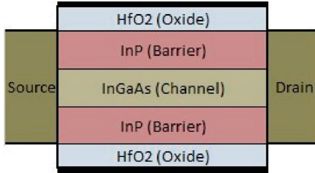
Fig. 9 Schematic diagram of the InGaAs/InP based DG MOS-HEMT
