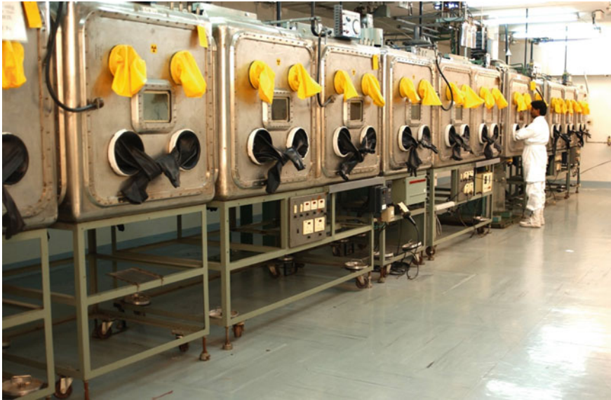
Fig. 3.2 Glove box train for fabrication of plutonium-bearing fuels
