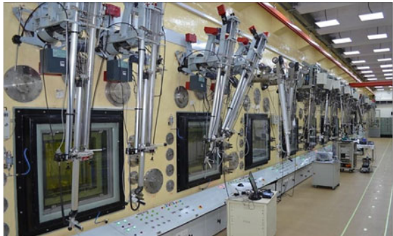
Fig. 6.4 Hot cell viewing windows and master–slave manipulators in the operating area of the hot cells [9]
