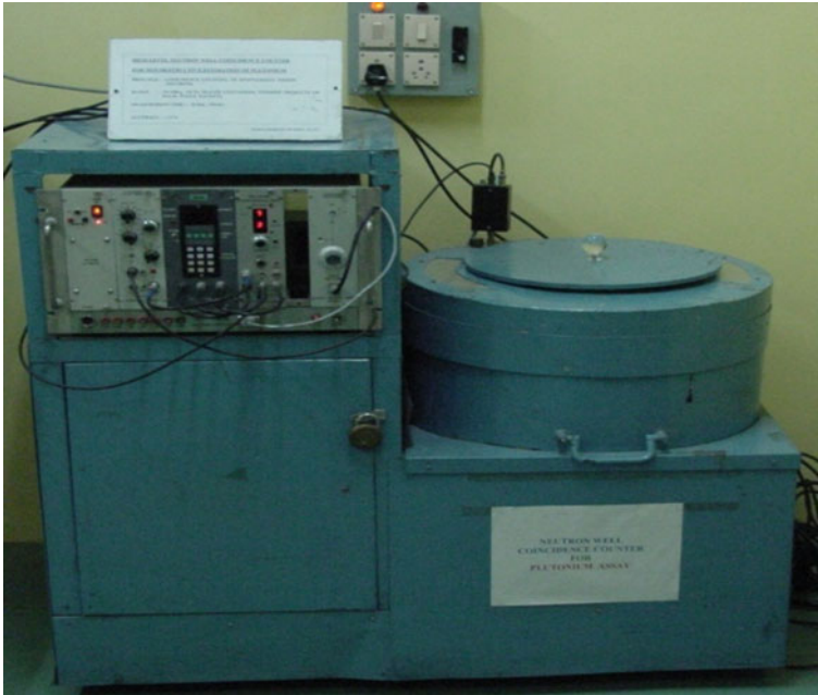
Fig. 9.4 Photograph of neutron well coincidence counter
