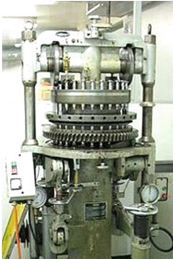
Fig. 3.4 Rotary press used for pelletization
