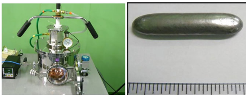
Fig. 2.19 Vacuum/inert arc melting setup (left) and Thorium metal finger (right)
