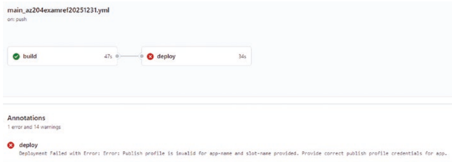
Figure 4-18. The slot has its own publish profile, so you must download that and store it in GitHub secrets
