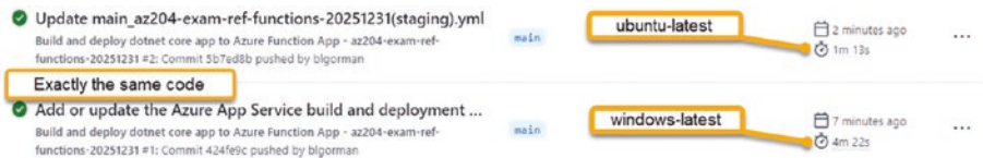
Figure 6-14. The Ubuntu agent is orders of magnitude faster than the Windows agent to build and deploy .NET to Azure
