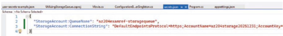
Figure 13-4. Ensuring the connection string and queue name are in your local secrets file
