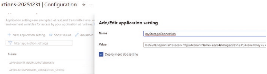
Figure 6-19. Make sure to set the connection string information for your Azure Storage Account where the file will be uploaded so the function app can connect to the storage account
