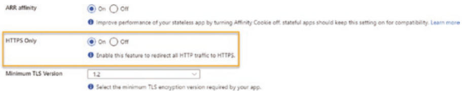
Figure 4-28. The remaining platform settings, with the interesting setting for HTTPS Only set to On
