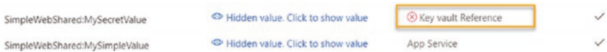
Figure 8-20. Access to the Key Vault secret is not configured correctly so the page shows a red X next to the Key Vault Reference
