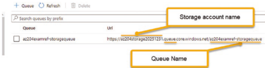
Figure 13-2. The full URL for the storage queue is shown. It may seem simple, but this is a critical part of working with the queue over HTTP/HTTPS should you desire to do so
