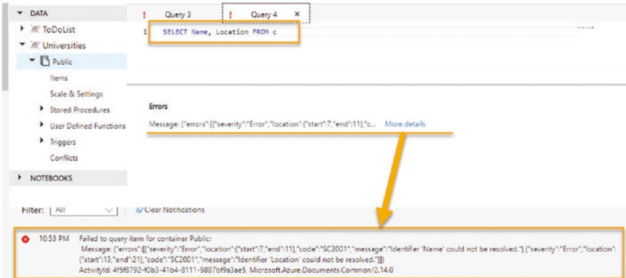
Figure 2-22. The Name and Location fields are stated to be unresolvable. This can be confusing since they are valid fields. The problem is the lack of the alias
