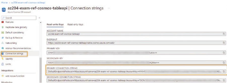
Figure 2-12. The connection string for the new Table API Cosmos Account is under the Connection String left-navigation menu item
