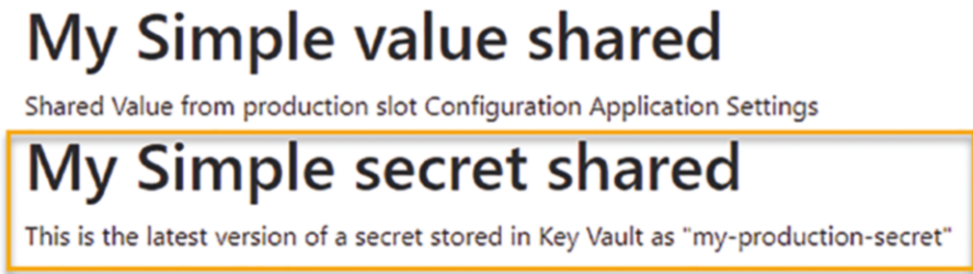
Figure 8-26. The value is retrieved from the Azure Key Vault once permissions and settings are configured without having to make any changes to code
