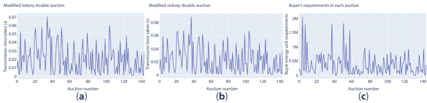
Figure 8.5 The total time taken for the proposed system to run is depicted along the x axis in Figures 8.5(a) and 8.5(b) for lottery and Vickrey double auctions respectively and the y axis represents the auction number. Figure 8.5(c) plots all the buyer energy unit requirements in each auction number from 1-144. This value remains the same for both types of markets. After taking the mean of all 144 values it was found that the program calculates results for lottery double auction in an average of 0.0186s and Vickrey double auction in 0.0216s.
