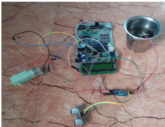
Figure 15.7 Hardware circuit of water management system.
