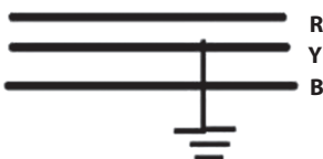
Figure 18.3 Double line-to-ground fault.
