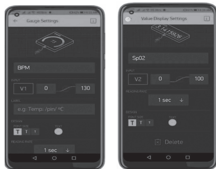
FIGURE 10.11(C) Setting up gauge and display widget.
