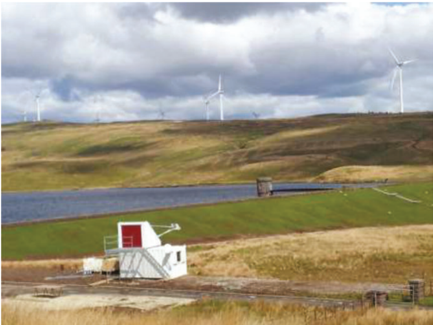
Figure 5.1 PoC planar HSR array in a trial of air surveillance in the presence of wind turbines
