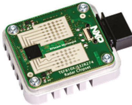
Figure 4.11 NXP TEF810x fully integrated 77 GHz transceiver
