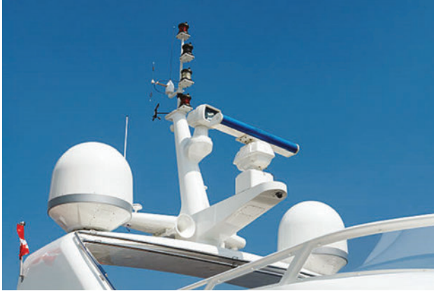
Figure 1.3 Maritime surveillance radar enabling the voyage data recording (VDR) system
