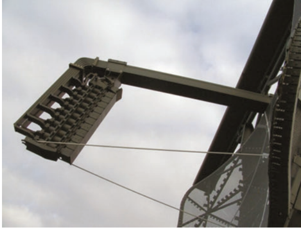
Figure 2.4 A 3-D mechanically scanned radar (courtesy CSIR)
