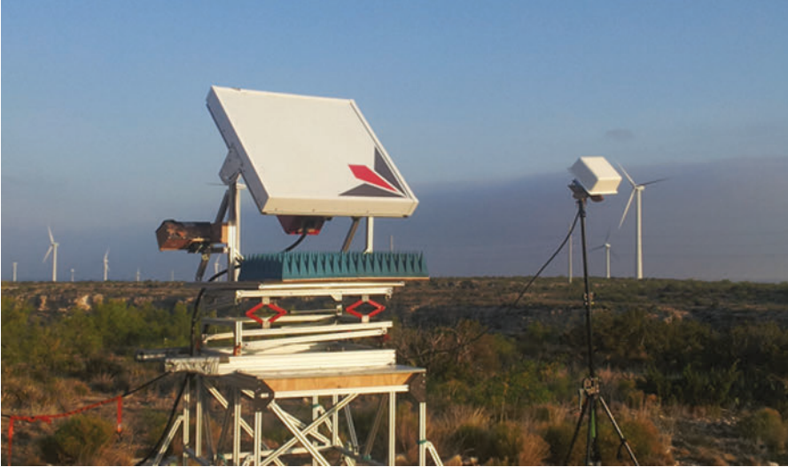
Figure 5.2 Proof of concept HSR in operation within a wind farm near Iraan, West Texas. The main enclosure houses the receiving array and the smaller radome houses the transmitter.
