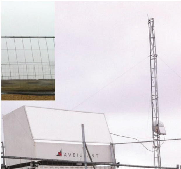
Figure 4.6 Aveillant Theia 64A on the beach at Muckleburgh, Norfolk, demonstrating mitigation of 80-turbine Sheringham Shoal wind farm
