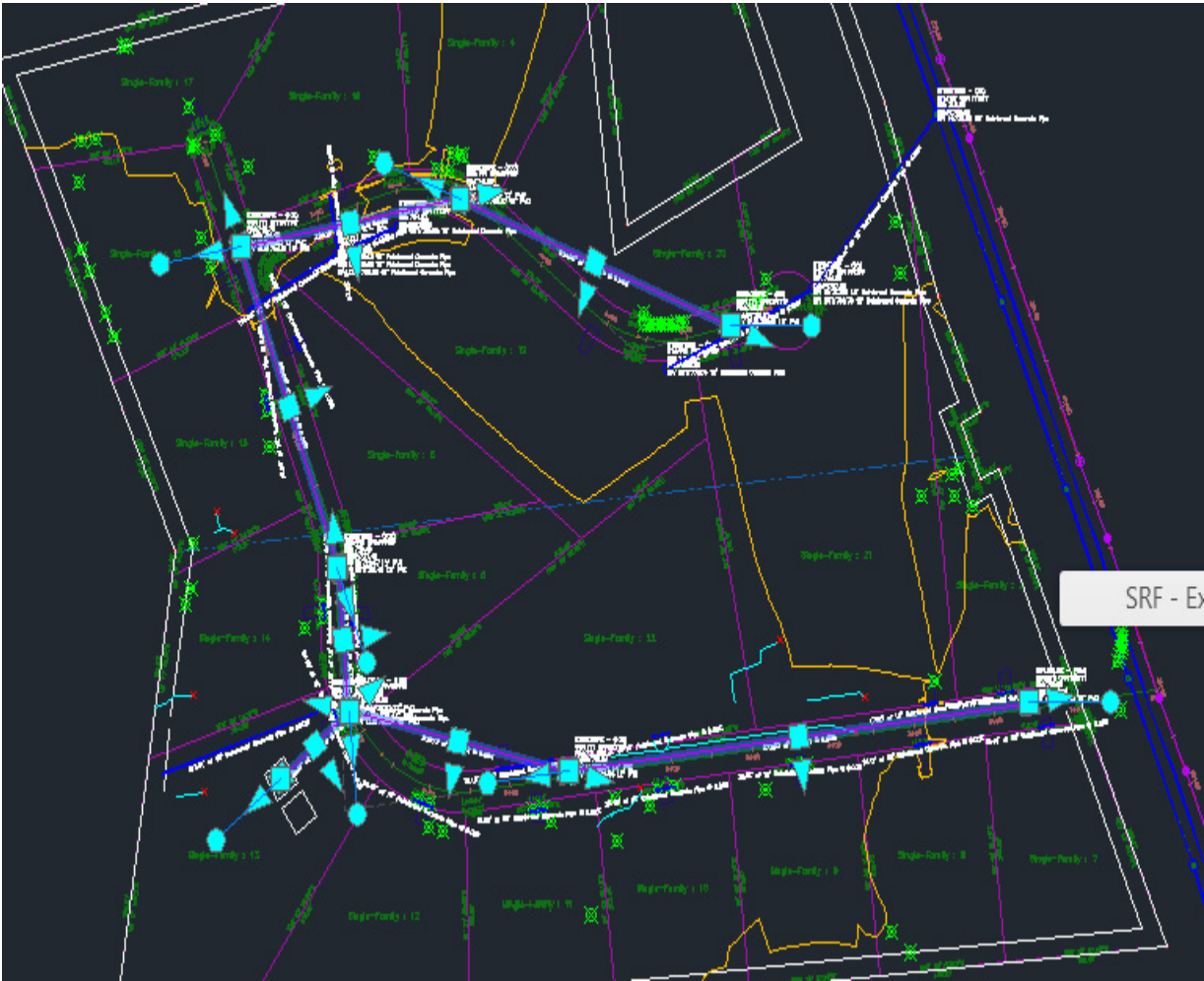
Figure 12.24 - GPN - Proposed Sanitary Sewer gravity utility network
