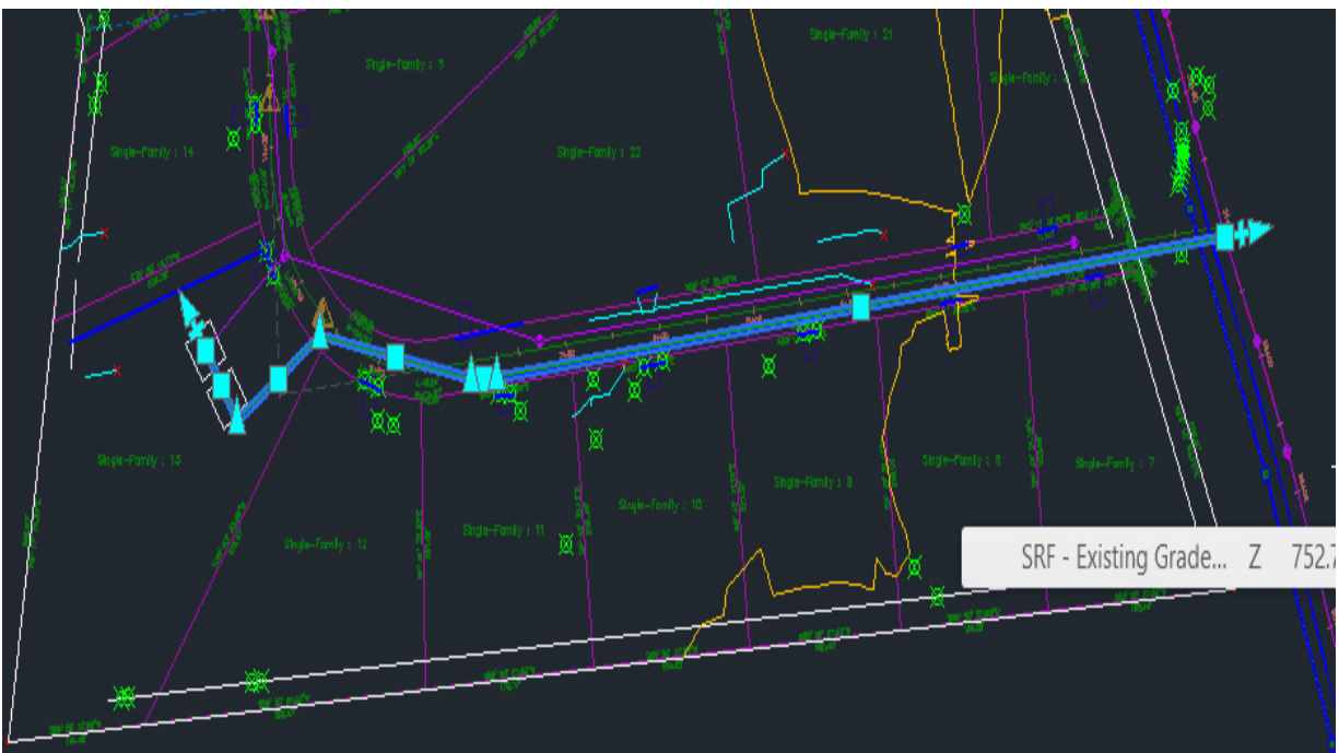
Figure 12.28 – Force main pipe run design
