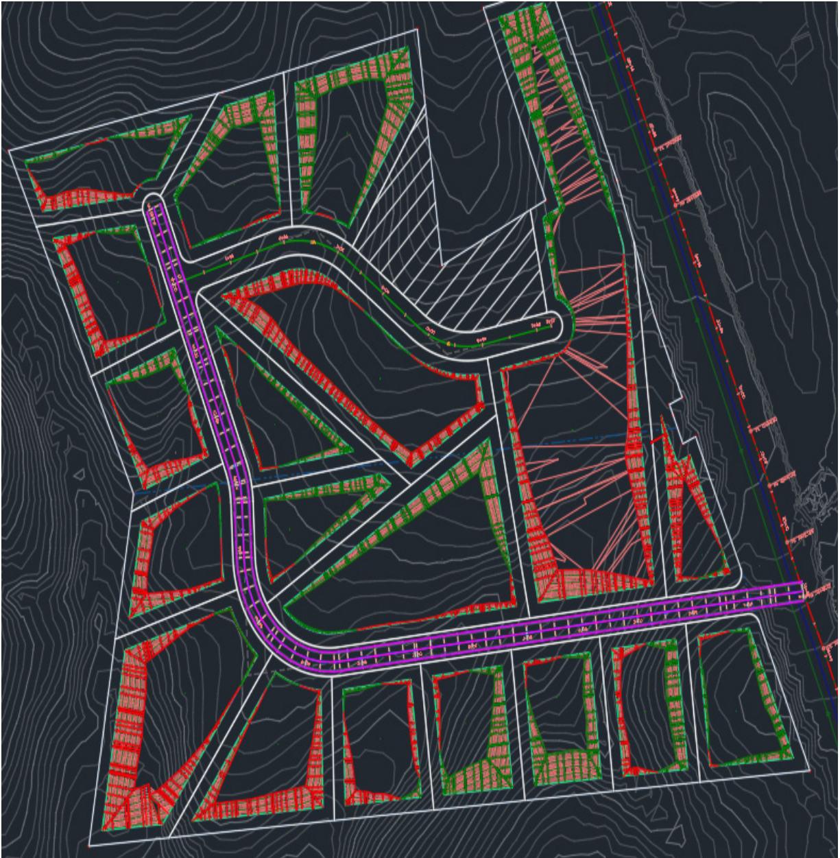
Figure 10.16 – Residential Subdivision for the first corridor model
