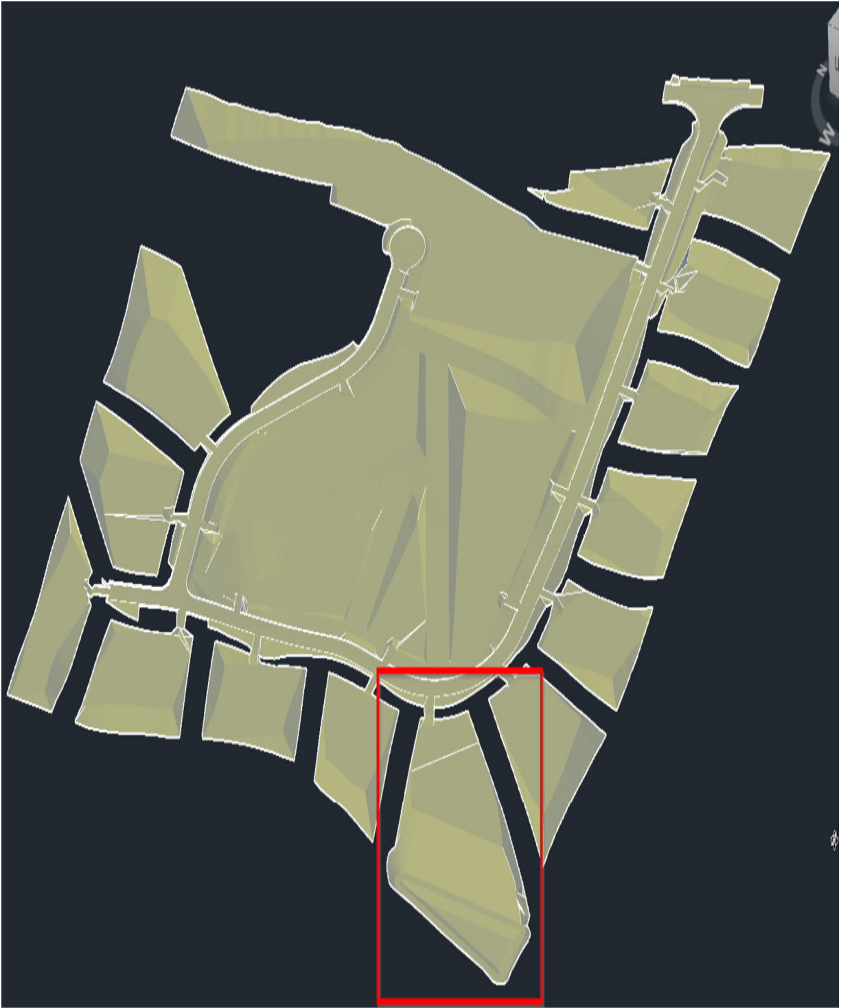
Figure 12.11 - Graded detention pond
