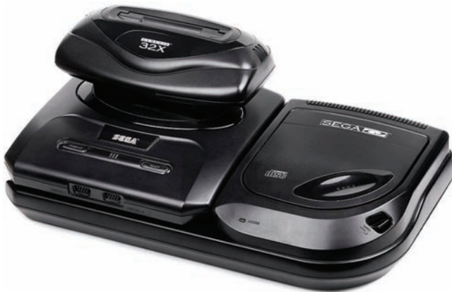
FIGURE 8.11 The Sega 32X on the top of a Model II Sega Genesis, on top of a Sega CD II.
