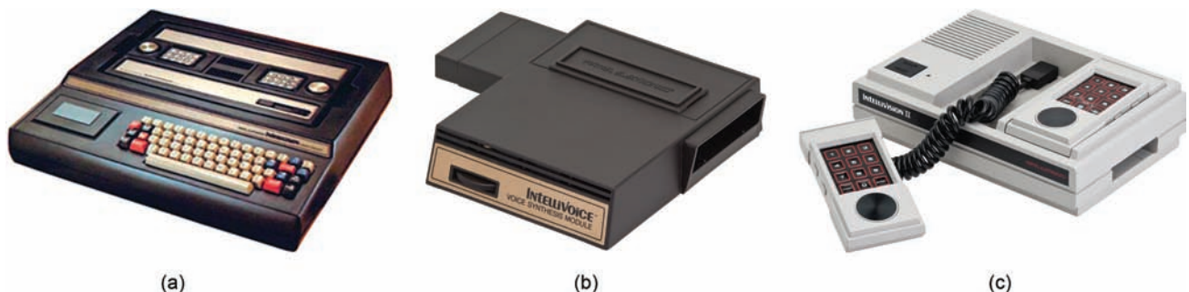
FIGURE 3.15 The Intellivision keyboard component (a), Intellivoice adapter (b), and Intellivision II console (c).
