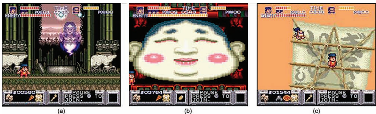
FIGURE 6.21 Screenshots from Konami’s The Legend of the Mystical Ninja displaying the Super Nintendo’s color layering (a) and Mode 7 scaling (b) and rotation (c) effects.
