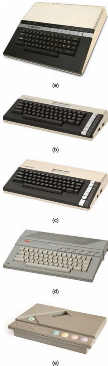
FIGURE 4.11 Evolution of the Atari 8-bit computers: (a) 1200XL, (b) 600XL, (c) 800XL, (d) 130EX, and (e) XEGS Game System.
