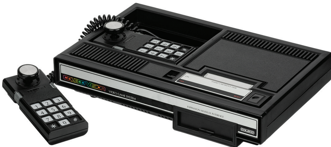
FIGURE 3.17 ColecoVision video game console with two joystick controllers.
