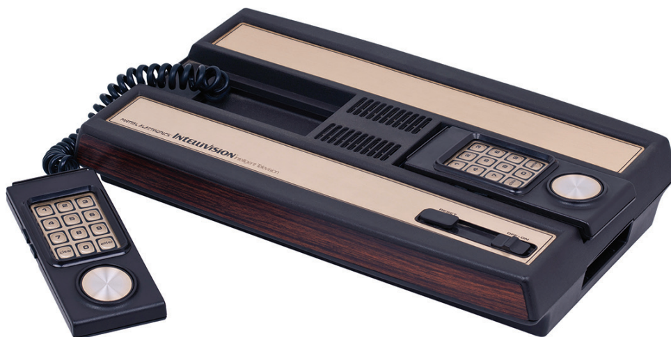
FIGURE 3.10 Mattel Intellivision with its controllers that could be stored inside the unit.
