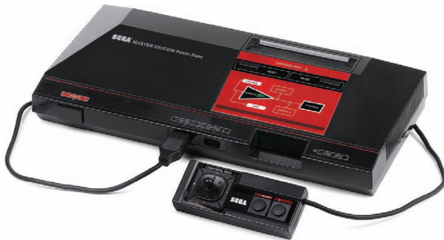
FIGURE 5.12 Sega Master System “Power Base” and D-Pad controller with joystick inserted.
