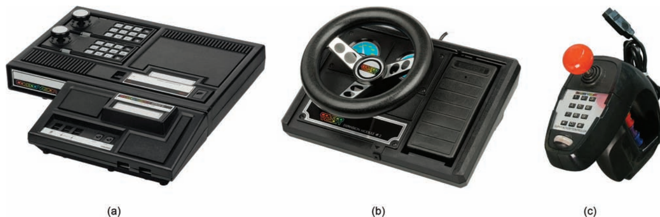
FIGURE 3.19 ColecoVision: (a) VCS adapter, (b) steering wheel, and (c) Super Action Controller.
