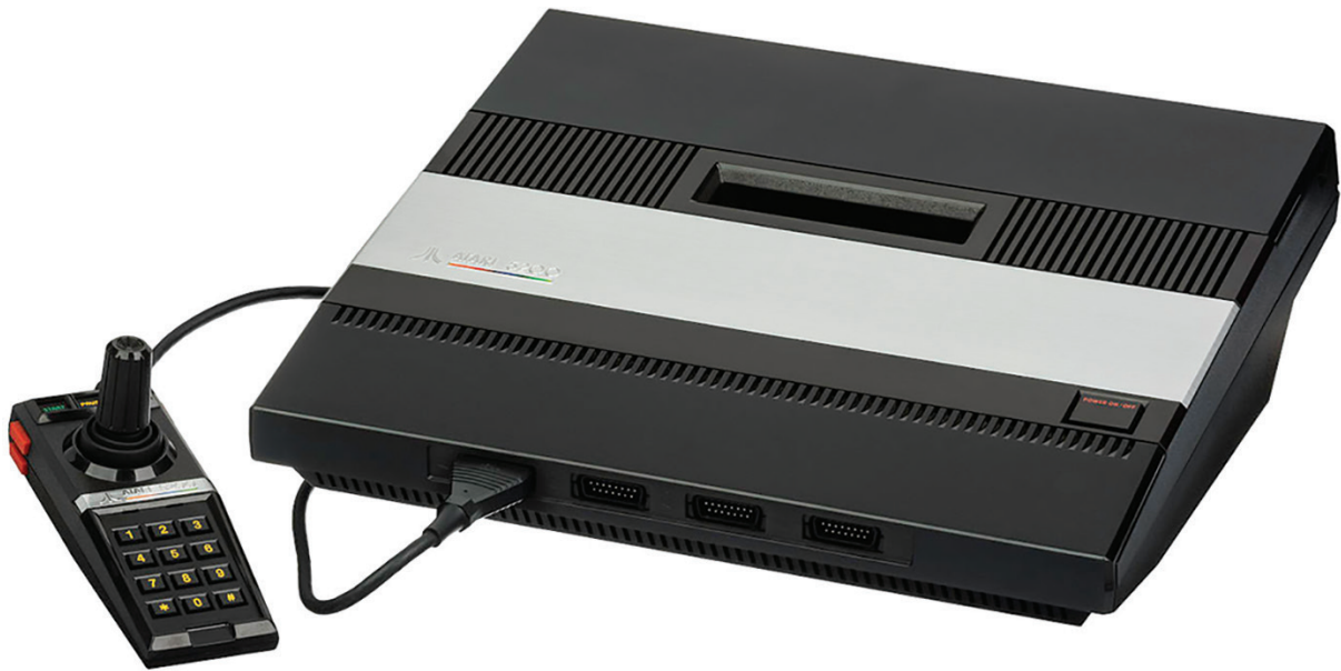
FIGURE 3.22 Atari 5200 with four controller ports and joystick controller.
