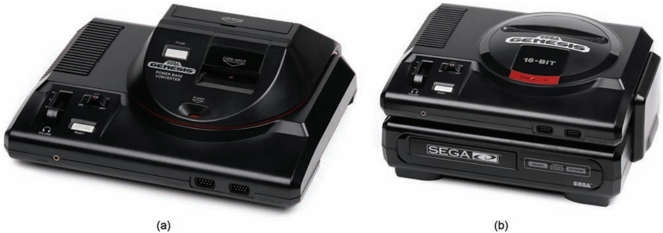
FIGURE 6.12 Two of the many Genesis add-ons: (a) Power Base Converter and (b) Sega CD.
