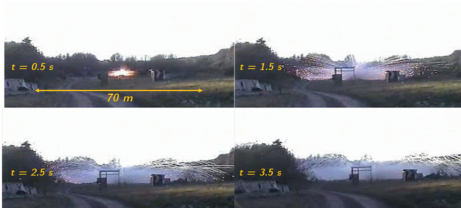
Figure D.7: Sequence showing the effect of detonative ignition of 700 g RP-based pyrotechnic obscurant.
