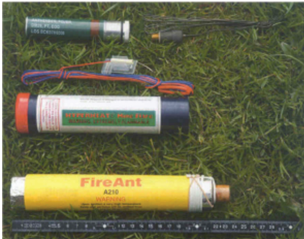
Figure M.6: Comparison of the sizes of the ignition charge and (thermite) flares used from top to bottom: DM29 ignition charge, fire, EOD, PT with igniter, electric, hyperheat mine flare with electric match, Fire-Ant A210 (from Kannenberger ).
