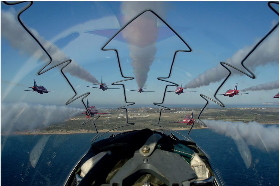
Figure D.3: Canopy of a BAE hawk showing the detonating cord WIKIPEDIA Capt. Alex Scott. https://commons.wikimedia.org/wiki/Category:Detonating_cord#/media/File:View_from_the_cockpit_of_a_Hawk_TMK1.jpg
