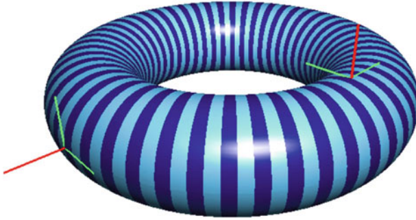
Fig. 7.18 The tangent vectors (green) and normal vector (red) on the left are for \theta = \phi = 0 . The vectors on the right are for \theta = \phi = \pi/2
