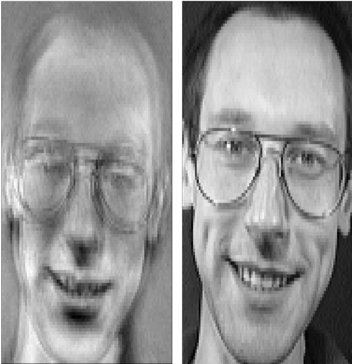
Figure 4-5. Extracted noisy face from a model inversion attack (left) and a training set image of the victim (right); the attacker is given only the person's name and access to a facial recognition system that returns a class confidence score
