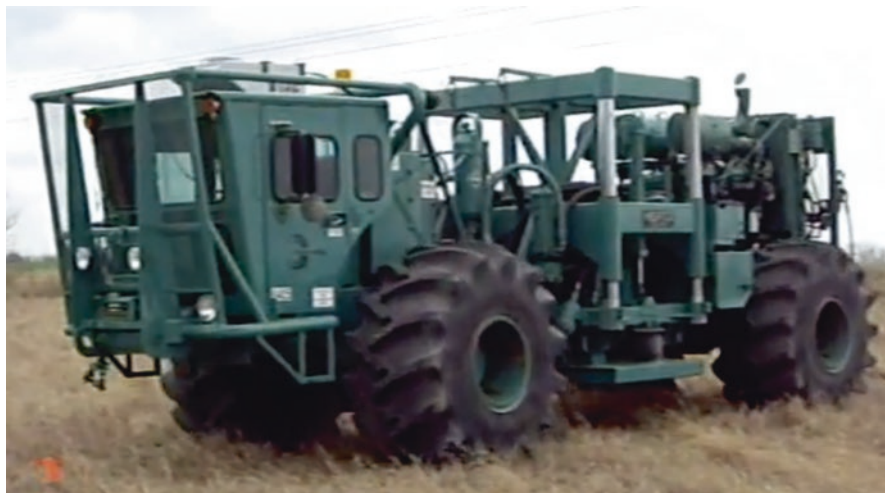
Fig. 1.6 Vibroseis truck with base plate (between tires) lifted for movement between shot points. (Photo credit: C. Liner)
