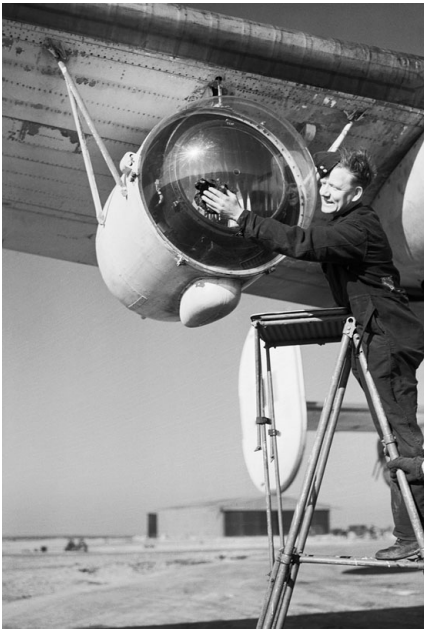
31 Another invention was the Leigh-Light, an ingenious weapon which used radar to track a U-boat on the surface at night, with a light that would only shine just as the aircraft was about to attack.
