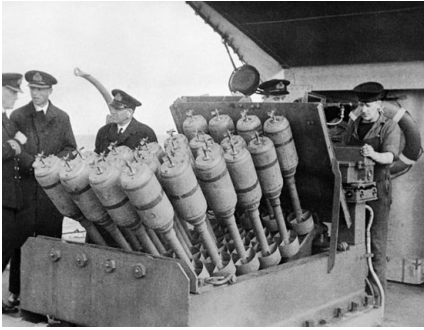
30 An example of British technical innovation was this forward-firing mortar, nicknamed Hedgehog, which first entered service in 1942.
