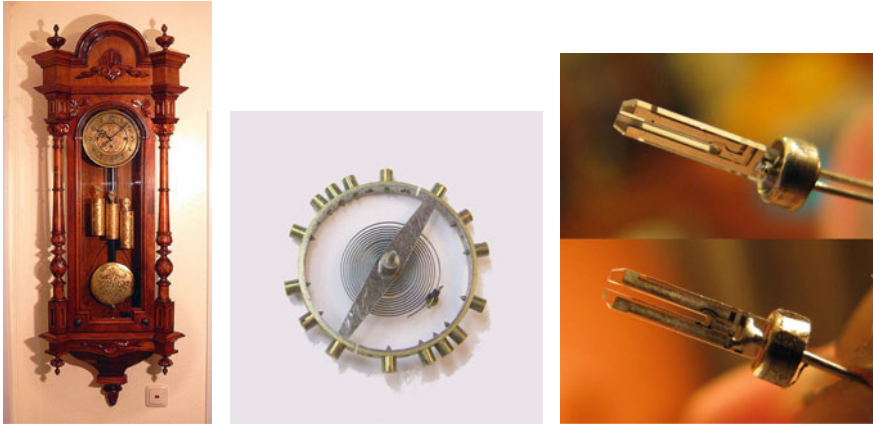
Fig. 9.5 Different types of clock oscillator. Left: Pendulum; Middle: Balance spring&wheel; Right: Quartz oscillator
