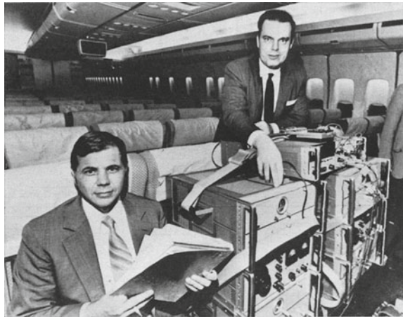
Fig. 9.25 Hafele (right) and Keating (left) carrying out their experiment with their atomic clocks
