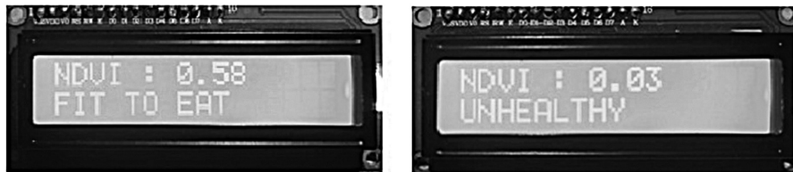
FIGURE 13.7 Calculated NDVI value of two different vegetables.
