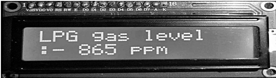
FIGURE 8.7(c) LPG gas levels of a sample having concentration of gas 865 ppm indicating no gas leakage status.
