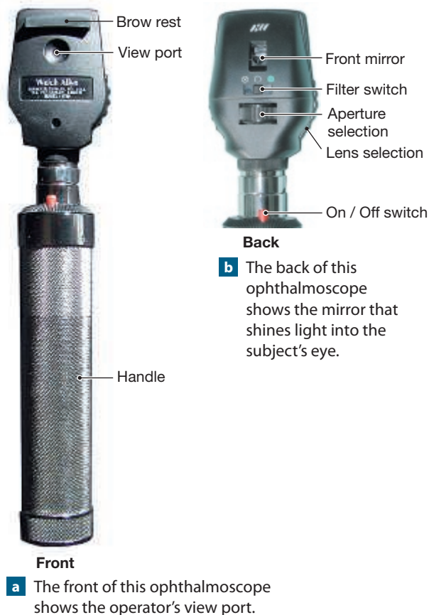
Figure 29.6 An Ophthalmoscope Internal structures of the eye are visible using an ophthalmoscope.
