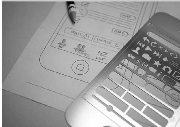
Figure 11-4: Using the iPhone stencil kit to draw your own mock-ups on paper.
