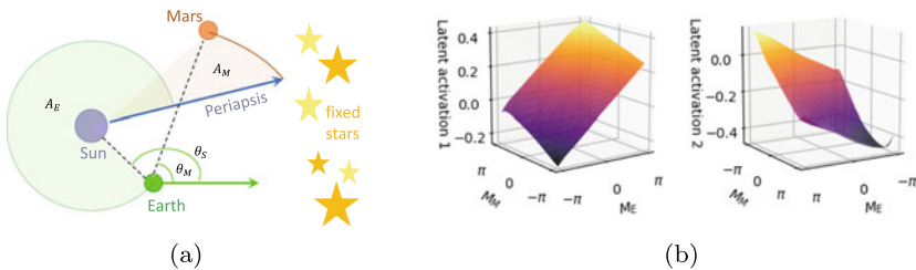
Fig. 10.9 Heliocentric model of the solar system. SciNet is given the angles of the Sun and Mars as seen from Earth at an initial time t_0 and has to predict these angles for later times. a Physical setting. The angles \theta_S and \theta_M of the Sun and Mars are observed from Earth (relative to the fixed star background). The areas A_E and A_M are swept out by a line segment joining Earth or Mars and the Sun, respectively. These areas are proportional to the mean anomalies M_E \propto A_E and M_M \propto A_M of Earth and Mars, respectively (see (10.1)). b Representation learned by SciNet . The activations r_{1,2} of the two latent neurons at time t_0 (see Fig. 9.3) are plotted as a function of the mean anomalies M_E and M_M . The plots show that the network stores and evolves parameters that are linear combinations of these heliocentric angles.
