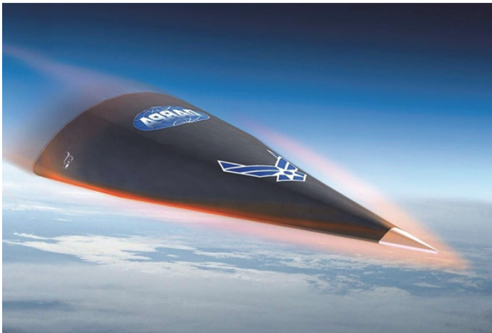
Fig. 1. Aero heating and ablation of HTV-2 in flight process.
